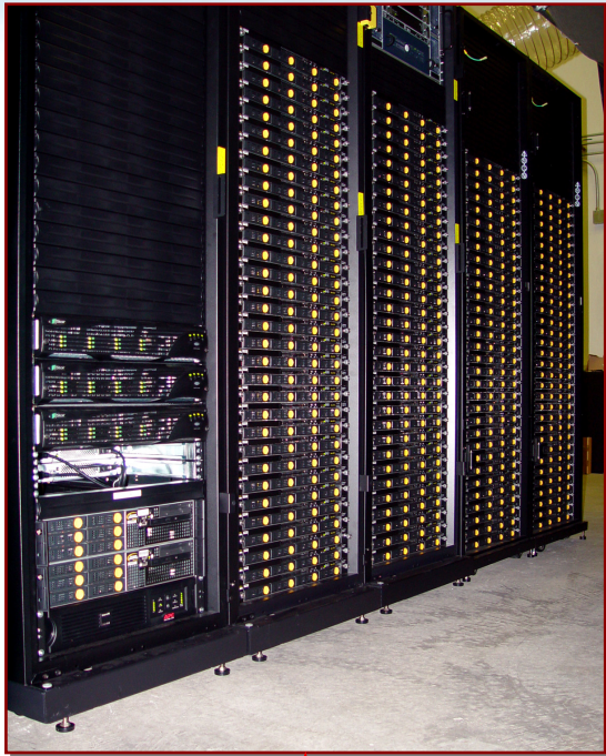
OVT System: 256 Opteron™ processors, InfiniBand, 10 terabytes NFS disk storage.
