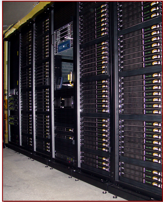
BES System: 284 Opteron™ processors, InfiniBand, 15 terabytes NFS disk storage.
