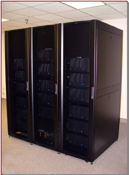
Visualization Cluster: 34 Opteron™ processors with high-end graphics cards, Gigabyte Ethernet, 50 terabyte parallel file system.
