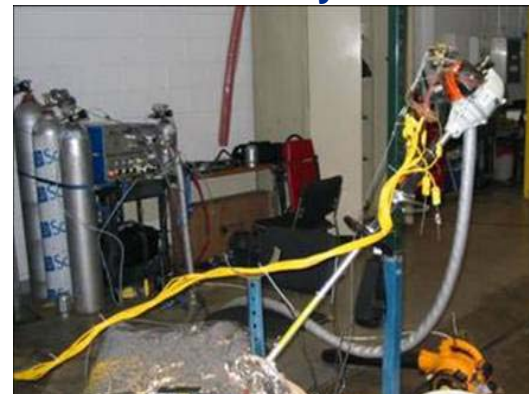
Raw Exhaust Sampling Via PEMS System
