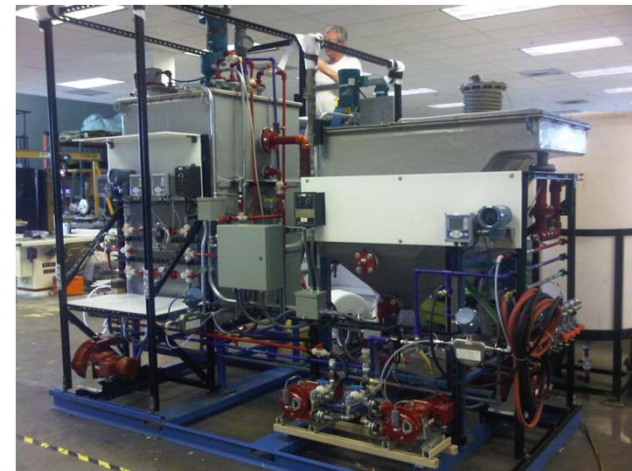
Simbol Materials: Lithium refining module. Built and tested in-house.
