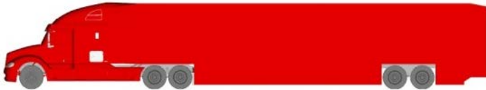
Gap Seal + Skirt + 32" Boattail (4-sided, hi)
