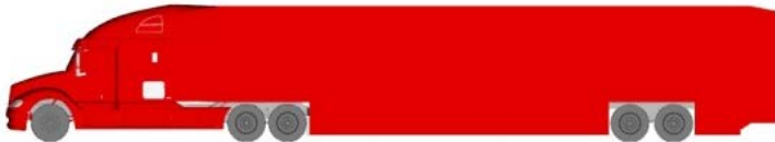
Gap Seal + Skirt + 32" Boattail (3-sided w/ base plate)
