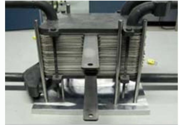
Planar SOFC (Courtesy of NexTech)
