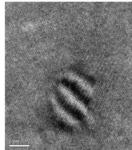
High resolution TEM image showing spinodally decomposed regions in PbTe-16%PbS.
