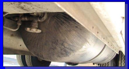
Typical installation in multiple vehicles of the same vintage •No shielding of exposed cylinder under vehicle •PRD on vertical cylinder isolated from cylinder exposure
