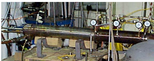
Figure 8. Phase II anode gas combustor (also known as a tail gas combustor, or TGC).
