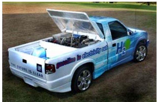
Chevrolet S-10 truck with on-board gasoline reformer.
