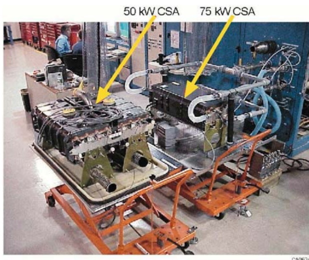
Figure 9. Advanced 75-kW power subsystem.
