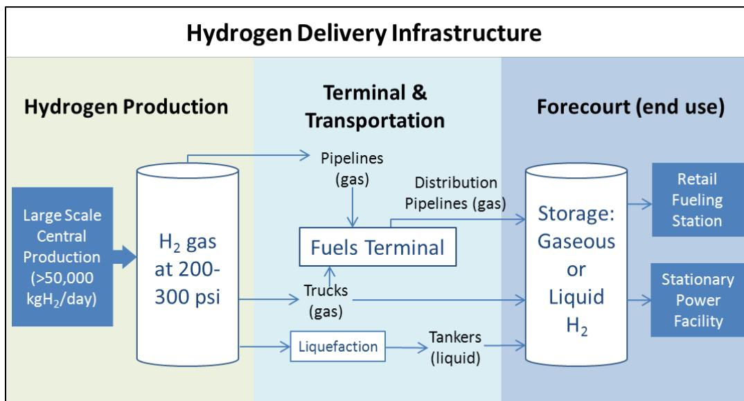
Figure 1. Hydrogen Delivery Scope
