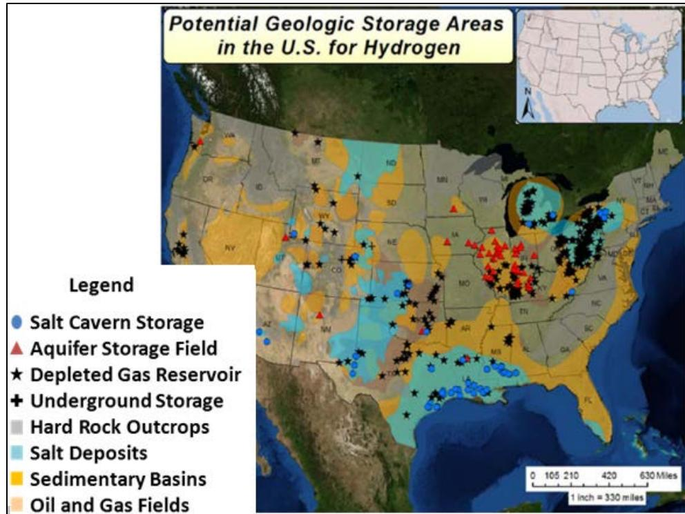
*Figure 9. Potential Geologic Storage Sites for Hydrogen in the United States*<sup>17</sup>
