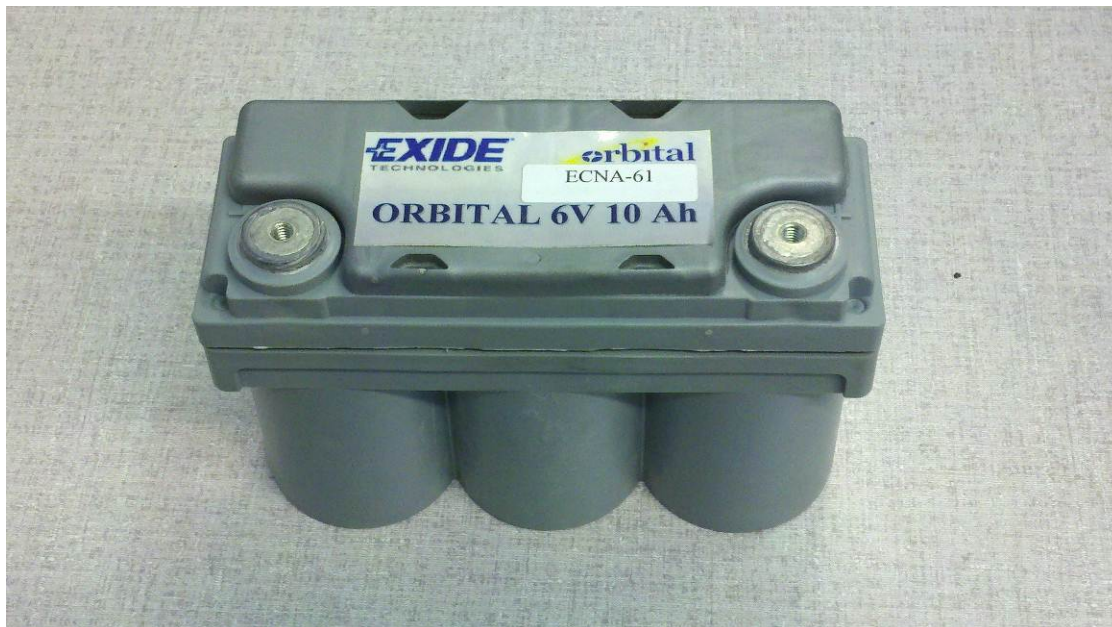
Figure 54. Picture of a 6-V, 10-Ah, Exide high-carbon battery.
