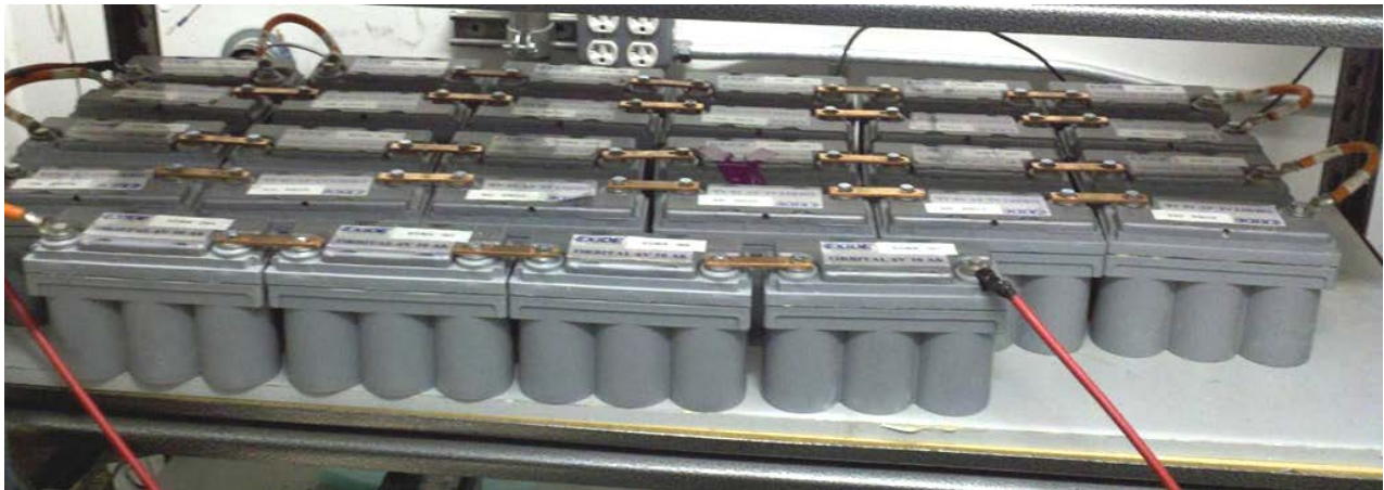
Figure 61. Picture of a vehicle-sized Exide pack cycling in the laboratory.
