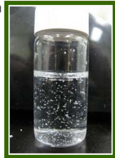
Example: NaCl encapsulated with Polystyrene and suspended in water (does not dissolve).
