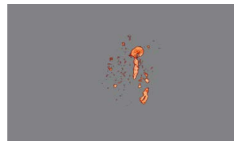
Lower threshold of CT reconstruction to isolate precipitate
