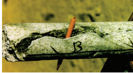
Figure 40. Typical fracture in geothermal production zone, which often produces total lost circulation
