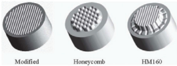
Figure 11. Various diamond-substrate interface configurations
