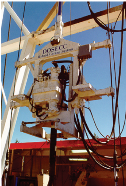
Figure 50. Hybrid coring system hanging in big-rig derrick at Long Valley, California
