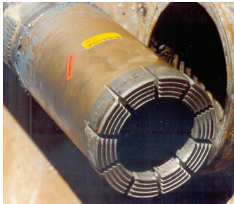
Figure 39. Diamond-impregnated core bit used in slimhole drilling
