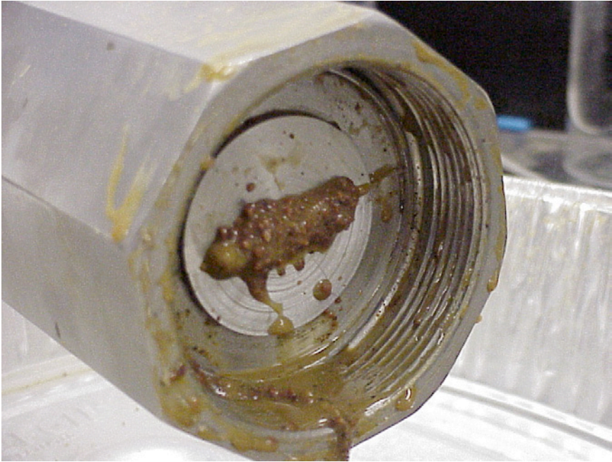
Figure 30. Slot plugged with lost circulation materials
