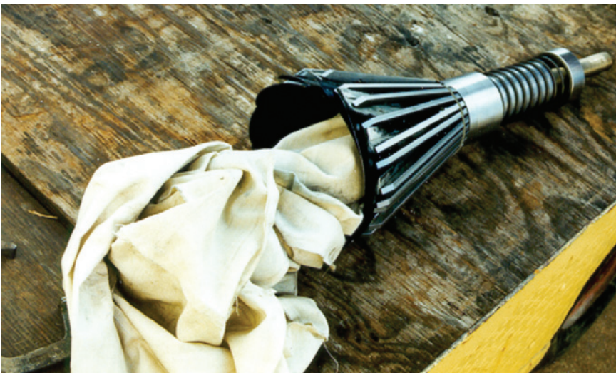
Figure 46. Petal-basket packer for The Geysers casing remediation
