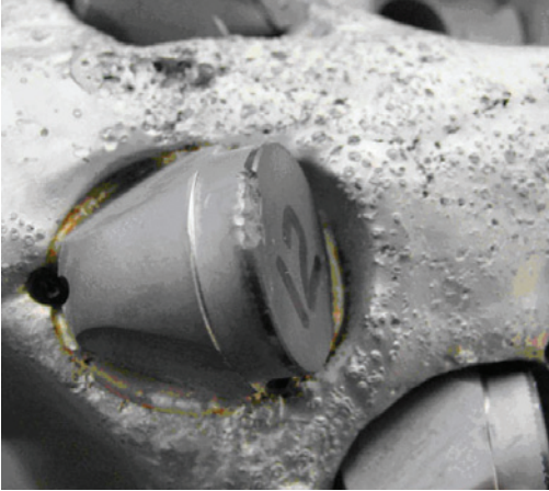
Figure 8. Worn PDC cutters in a drag bit
