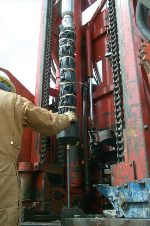
Figure 33. Packer with stinger ready to run in hole
