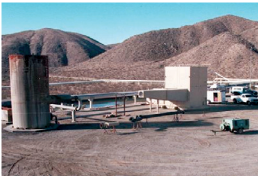
Figure 47. Low Emission Atmospheric Metering Separator on the right; conventional cyclone separator on the left
