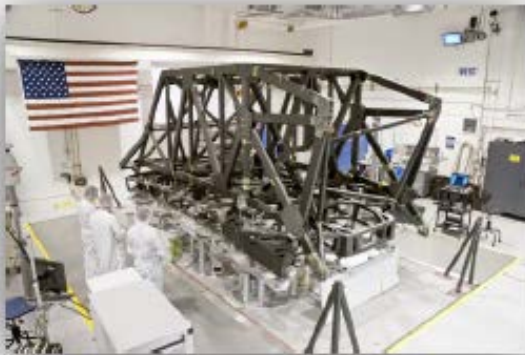
James Webb Space Telescope Primary Mirror Backplane Structure
