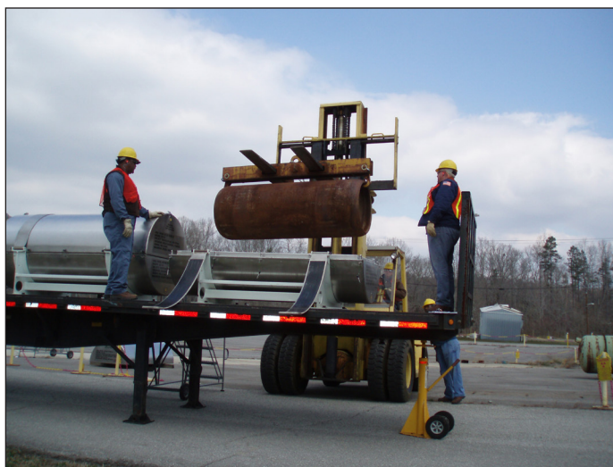
UF_6 cylinder being loaded for transport at ETPP
