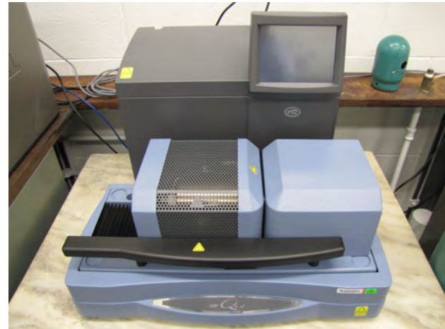
SDT-Q600 calorimeter, continuous weight change monitored weight ± 0.0001 mg
