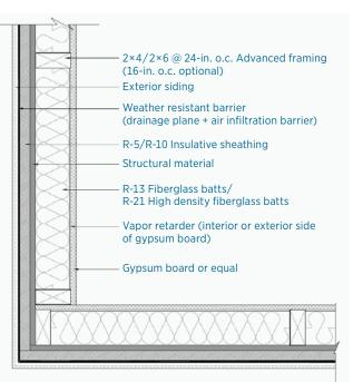
The figure to the left shows a typical wall section of a stud wall with exterior insulation. The design is intended to conform to the thermal requirements of the 2012 IECC for climate zones 5 (R-13+5), 6, 7, and 8 (R-13+10 or R-21+5).
