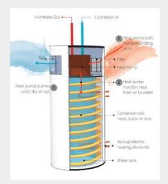
The most common arrangement of current HPWHs is an integrated water heater with a wraparound condenser and two backup electric elements. The figure above describes the typical components and operation of modern HPWHs in the U.S. market. Among the systems evaluated in this study, the only model to deviate from this configuration is the Stiebel Eltron unit, which has only one smaller (1.7 kW) upper element and always operates in hybrid mode.
