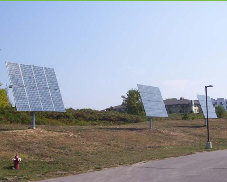
One of the first city-owned PV tracking systems is on the East Police Parking Lot. Tracking systems are built to move throughout the day to follow the sun's path, increasing electricity production. *Photo from The City of Madison, NREL/PIX 18355*
