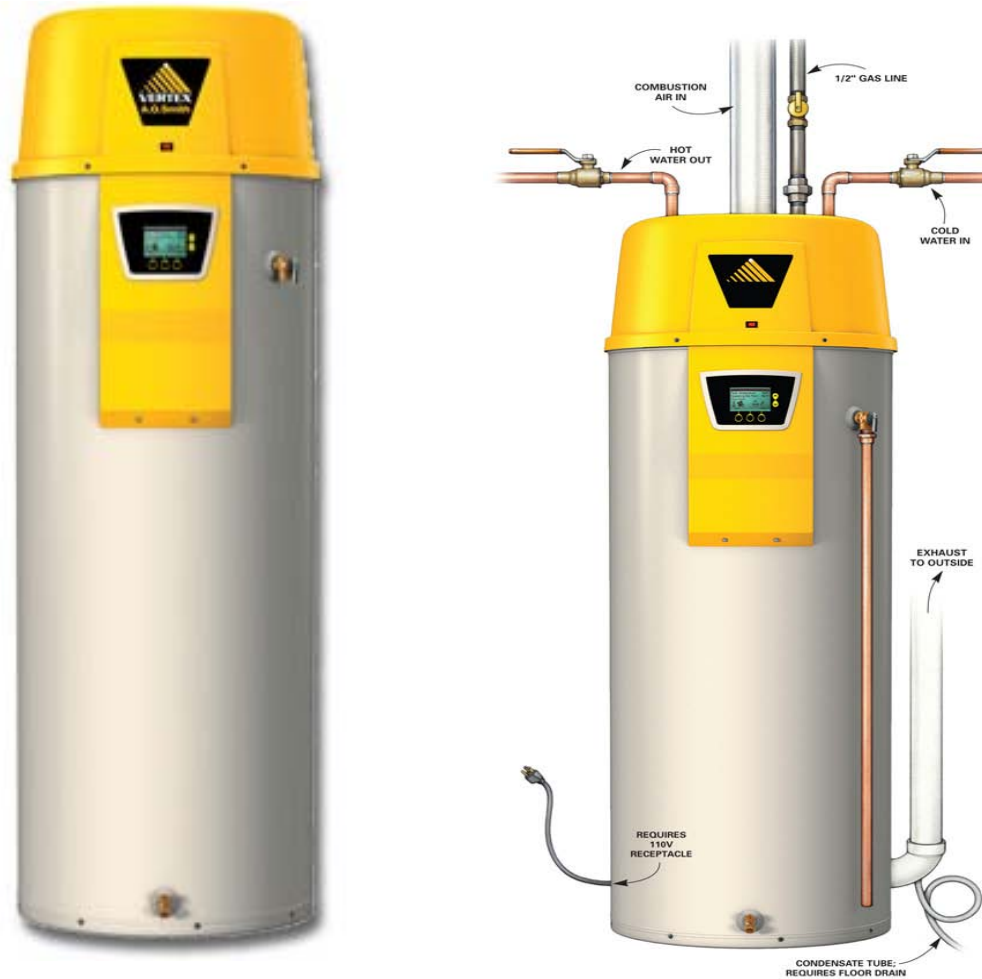
Condensing Gas-Fired Storage Tank
