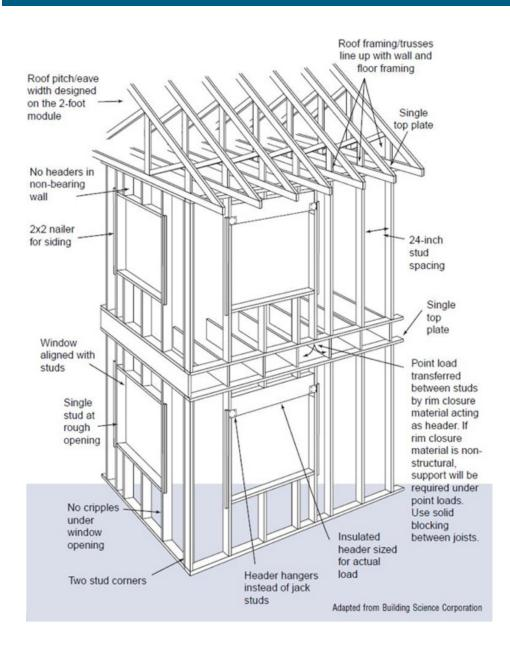
This drawing shows many aspects of advanced framing, including alignment of wall, ceiling, and floor studs on a two-foot grid, which requires planning to implement but yields significant material savings since most sheet goods are sold in two-foot increments.
