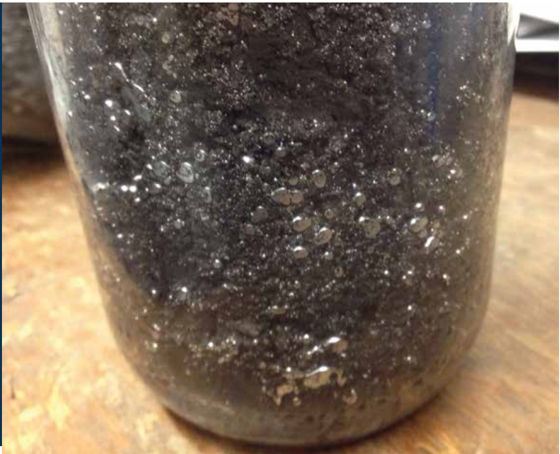
Mercury recovered from a contaminated tank
