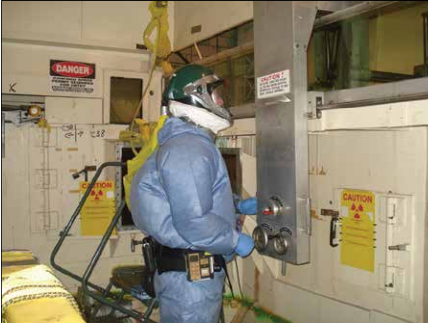
A worker in 3038 uses a glove box to package and dispose of waste
