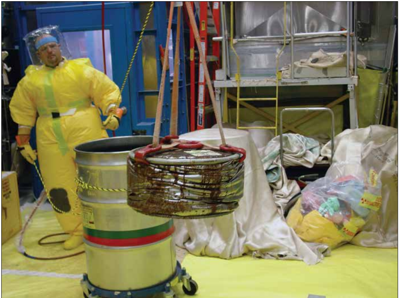
A TWPC worker removes a supercompacted waste puck from a 55-gallon waste drum
