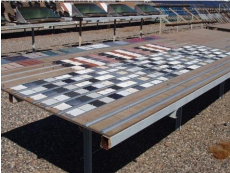
Sample 1: White Single-Ply Membrane, 5 Degree Tilt
