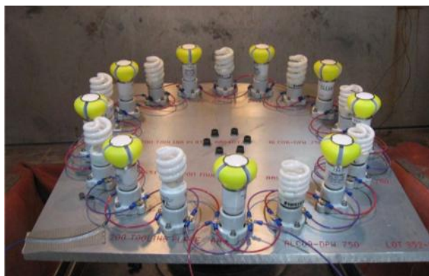
Stress testing of LED replacement lamps
