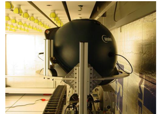
PNNL Test Apparatus for long term testing of LED replacement lamps
