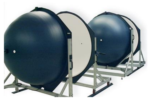
Integrating spheres used in LM-79 testing
