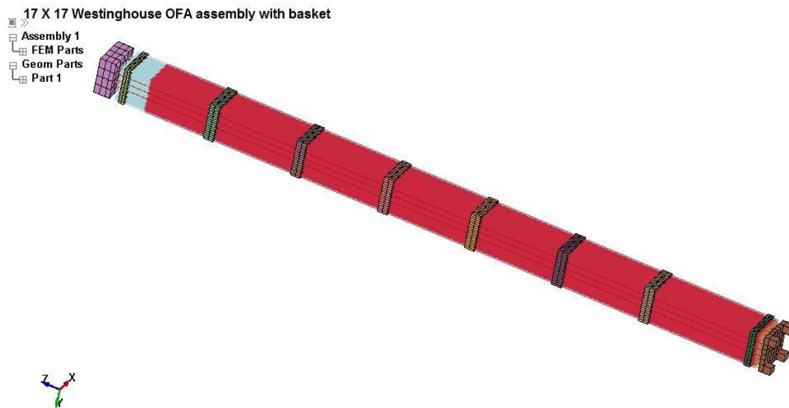
Figure 6.5. WE 17×17 OFA PWR Fuel Assembly Submodel (w/o Control Components)
