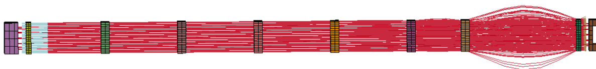
Figure 8.59. Fuel Rod Modal Deformation Shown on the Alternate Spacer Grid Design Case for the Sensitivity Analysis
