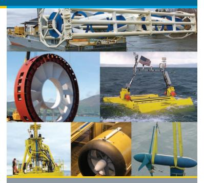
Marine and hydrokinetic devices include (clockwise from the top) Ocean Renewable Power Company's Turbine Generator Unit, NREL/PIX 17210; Columbia Power Technology's SeaRay, NREL/PIX 19381; Verdant Power's Free Flow System, NREL/PIX 17209; Free Flow Power Corporation's SmarTurbine, NREL/PIX 19382; the Wavebob point absorber, NREL/PIX 19384; OpenHydro's Open-Centre Turbine, NREL/PIX 19383
