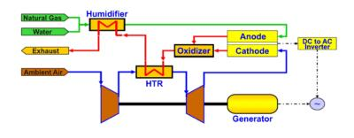
A schematic of a high-temperature fuel cell with a high-temperature recuperator (HTR)
