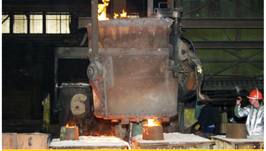
Harrison Steel facility where ductile iron is poured into casting molds
