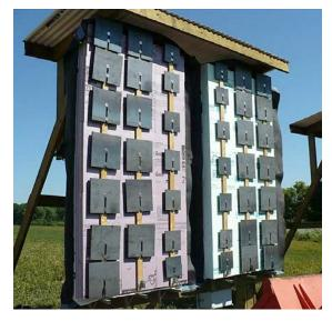
Exterior environmental exposure testing examined four types of insulation materials. Each test panel was constructed with two layers of 2-in. thick insulation and loaded to three different load magnitudes (8 pounds [lbs], 15 lbs, and 30 lbs per fastener). Researchers recorded the downward and upward vertical movement of the furring strips over a period of about 70 days. Daily movements were on the order of ±1/32 of an inch.
