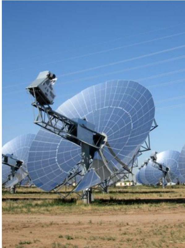
Figure A-5. The Stirling Energy System's SunCatcher, a 20-KW dish/engine CSP system with a Stirling engine
