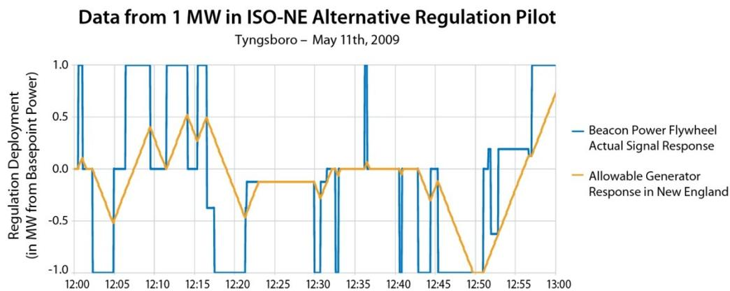
**Figure C-14. Fast-response flywheel storage providing frequency regulation**
