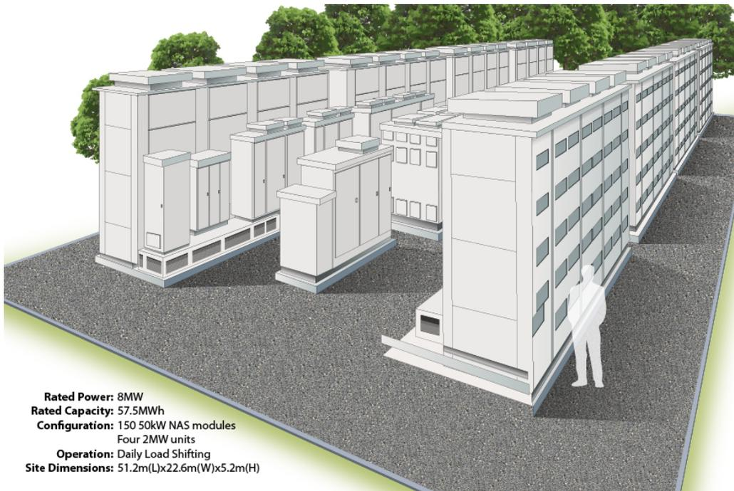
**Figure C-4. Layout of 8-MW NaS battery system**
