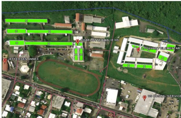
**Figure 5-1. Roof area survey screen shot, St. Thomas, with potential PV locations identified in green**
