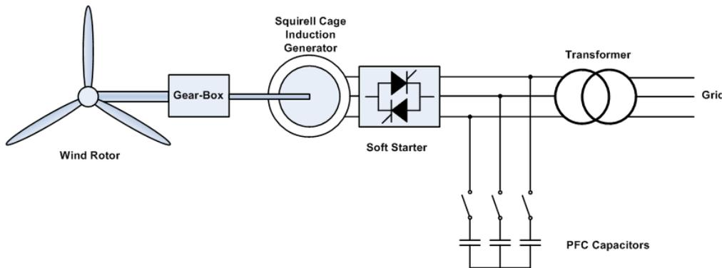
Figure A-1. Type 1 wind turbine
