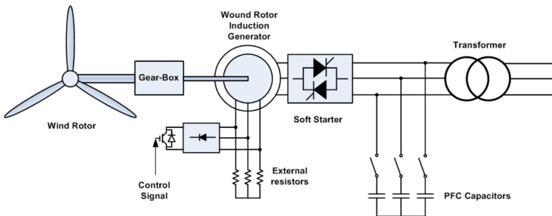
Figure A-2. Type 2 wind turbine
