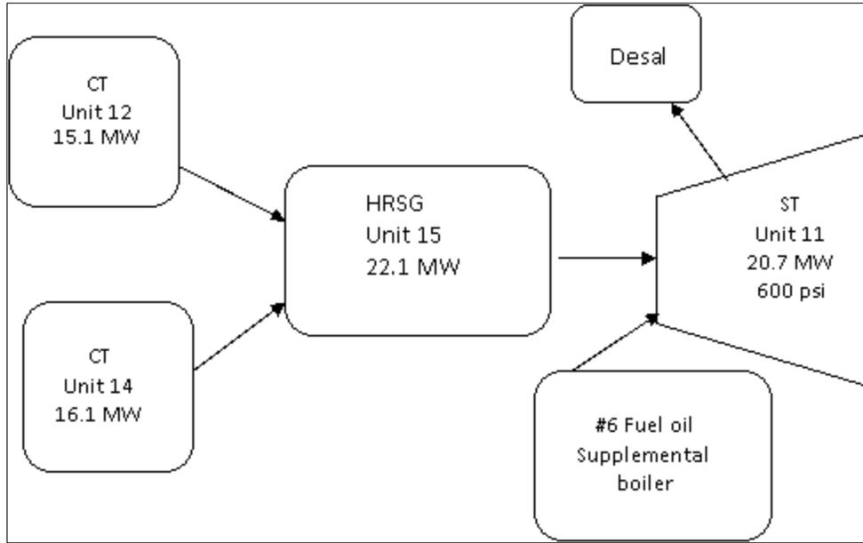
**Figure 4-7. Typical configuration for steam turbine #11**
