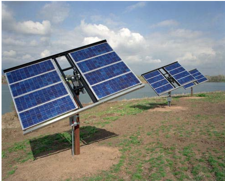
Figure 3. Typical one or two-axis tracking, flat-plate PV system (J. Thornton)
