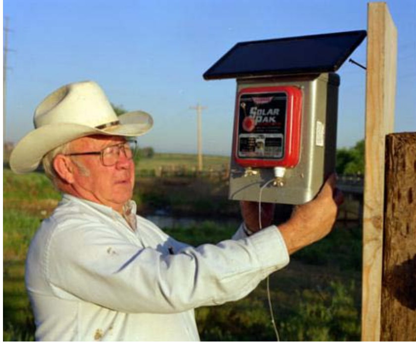
Figure 8. A PV-powered electric fence charger (NREL PIX 04347)
