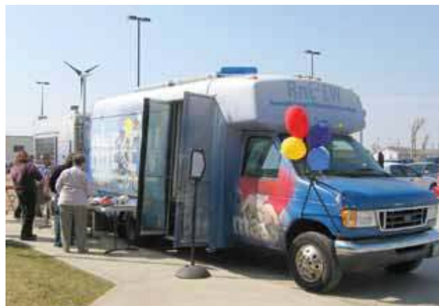
Figure 27. The RnE 2 EW vehicle is designed to take renewable energy technologies on the road. The vehicle is equipped with solar panels and a wind turbine, which produce enough power to run everything that requires energy during an educational event like this one in Greensburg.
