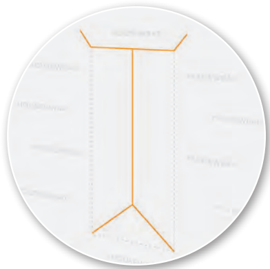
STEP 2 Cut modified "I" in housewrap
