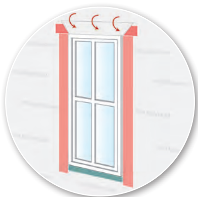
STEP 8 Fold down head housewrap.
