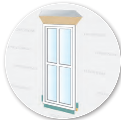
STEP 6 Install window; plumb, level, and square as per manufacturer's instructions.
