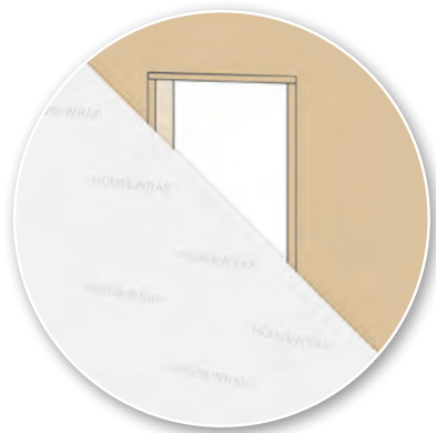
STEP 1 Install OSB and housewrap on wood frame wall.
