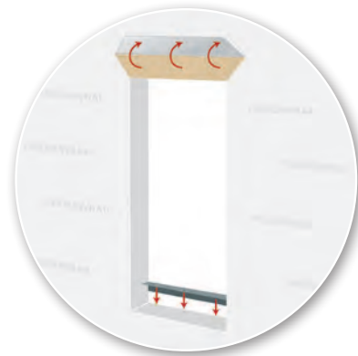
STEP 3 Fold housewrap in at jambs and sill. Temporarily fold up housewrap at head. Install backdam.
