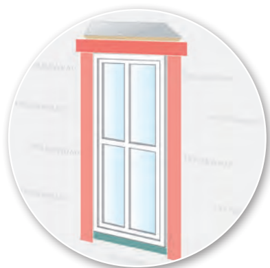
STEP 7 Install jamb flashing first; install a drip cap (if applicable); install head flashing.
