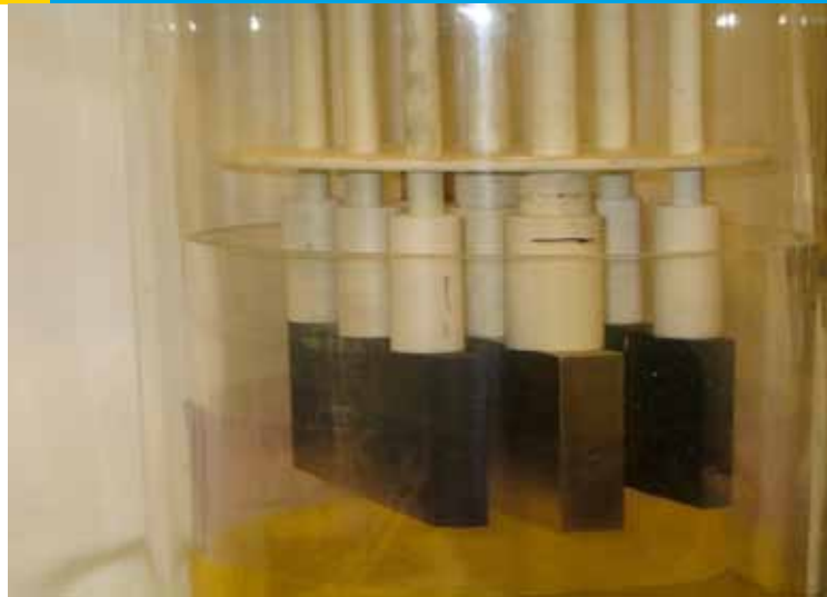
Laboratory-scale ultrahigh-efficiency aluminum production cell, showing the arrangement of a central metal anode and wetted cathodes.
