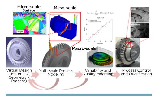
Multi-scale modeling tools for enabling manufacturing-informed design. Photo courtesy of Third Wave Systems
