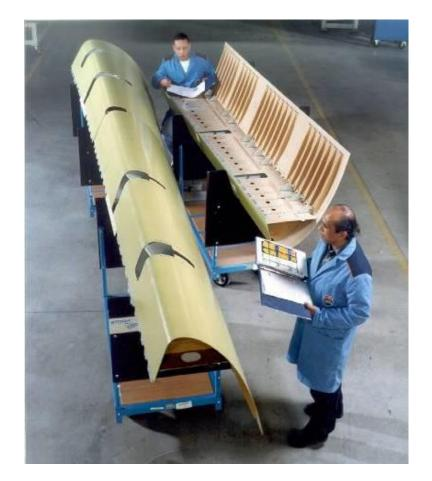
PPS – glass fabric composite fixed wing leading edge --- on Airbus A340 and A380
