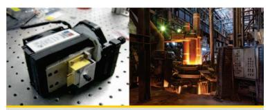
The Los Gatos Research mid-infrared laser module contains a quantum cascade laser mounted on a thermo-electric cooler (left). The Small Business Innovation Research (SBIR) Phase III analyzers will be deployed for long-term testing under industrial conditions at EAF facilities (right).
