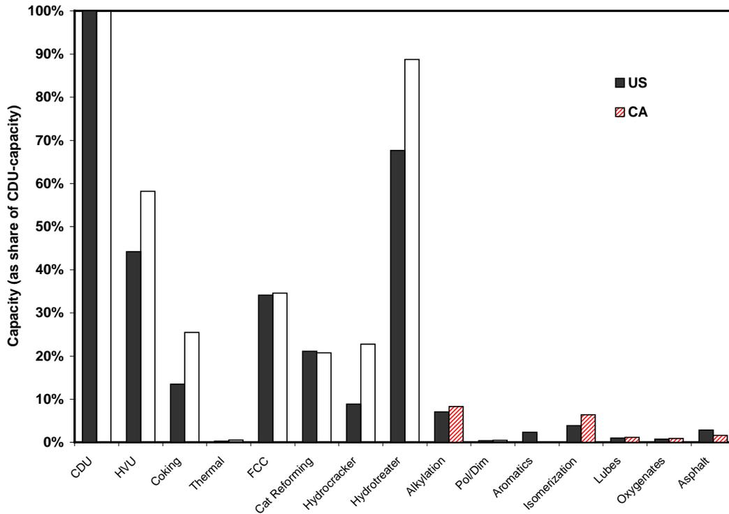
Figure 12. Capacity distribution of the major refining processes in U.S. and Californian petroleum refineries, expressed as share of installed CDU capacity, as of January 1<sup>st</sup>, 2003. Source: Oil & Gas Journal (2002).
