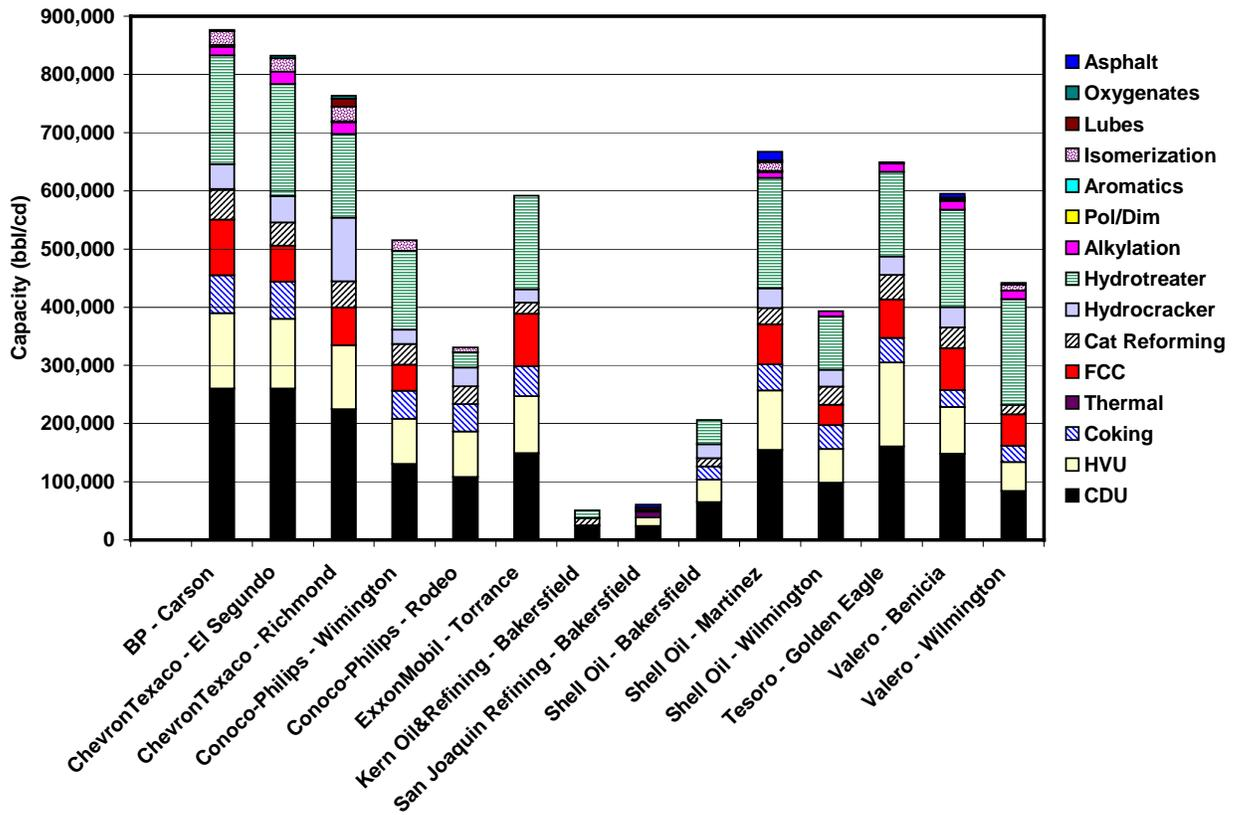
Figure 13. Process breakdown for the 14 operating refineries in California (as of January 1<sup>st</sup>, 2003), expressed as capacity (bbl/calendar day). Source: Oil & Gas Journal.
