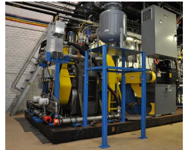
3.0-L single-cylinder engine installation
