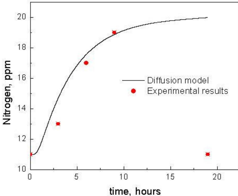
Figure 19, Nitrogen transport through slag layer, calculated and experimental, Trial 4
