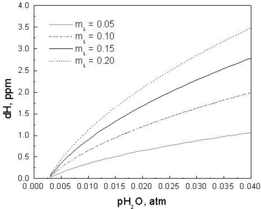
Figure 26, Hydrogen pickup for different mass transfer coefficients,  $H_i=3\text{ppm}$ ,  $\%S = 0.02$ ,  $h_o = 0.05$
