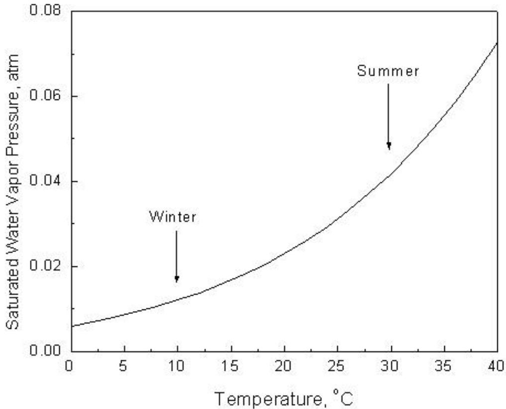
Figure 20, Water vapor partial pressure as a function of temperature [8]
