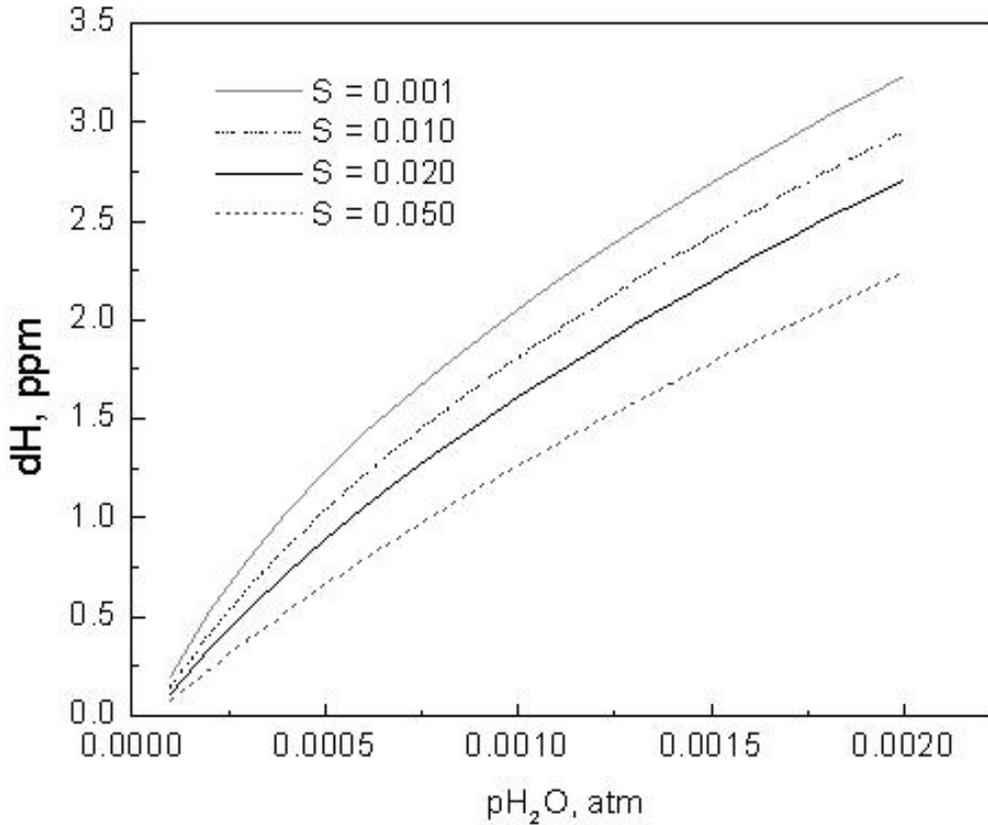
Figure 24, Hydrogen pickup for different sulfur concentrations at the bubble surface,  $H_i=3\text{ppm}$ ,  $h_o = 0.001$ ,  $m_L = 0.097 \text{ cm s}^{-1}$
