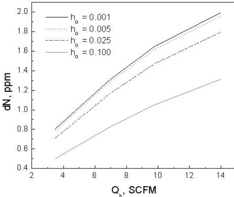
Figure 27, Nitrogen pickup at the spout eye for different oxygen activities, N<sub>i</sub> = 10 ppm, % S = 0.005, stirring time = 20 minutes and slag thickness = 5 cm
