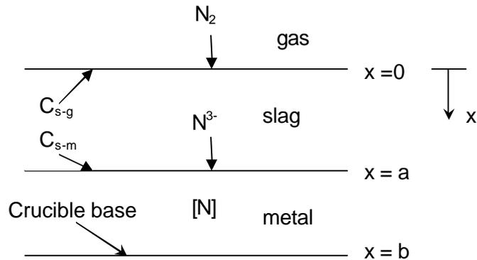
Figure 14, Schematic representation of the nitrogen diffusion through the slag layer
