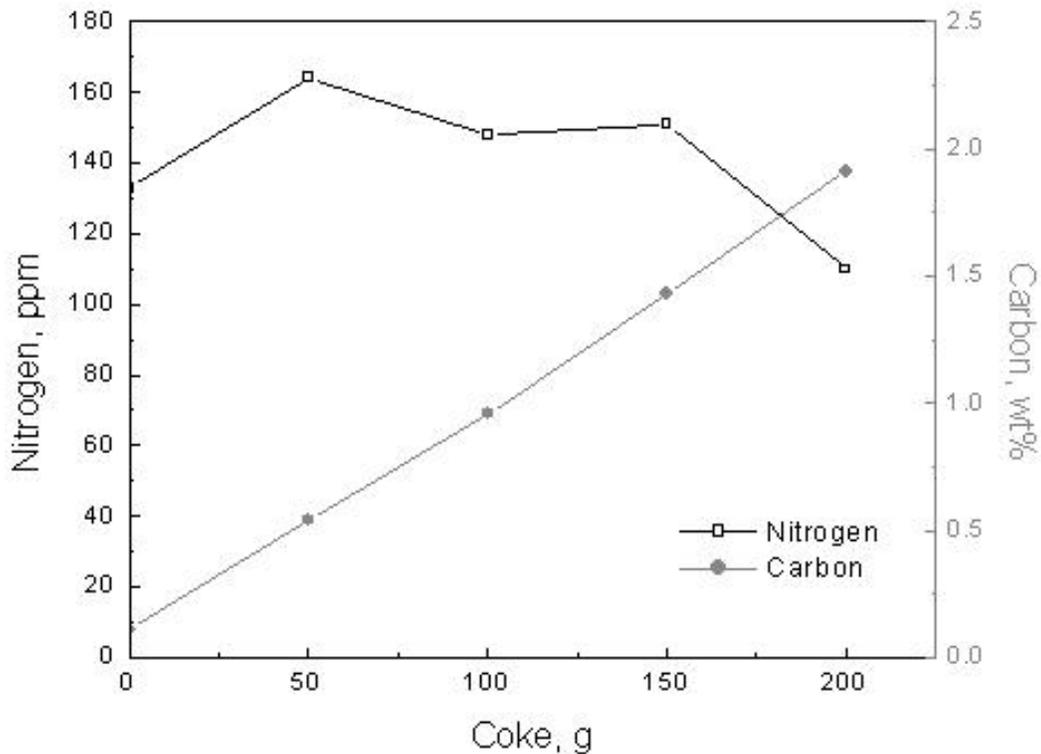
Figure 6, Effect of pitch coke addition on the nitrogen and carbon content of iron, Trial 1
