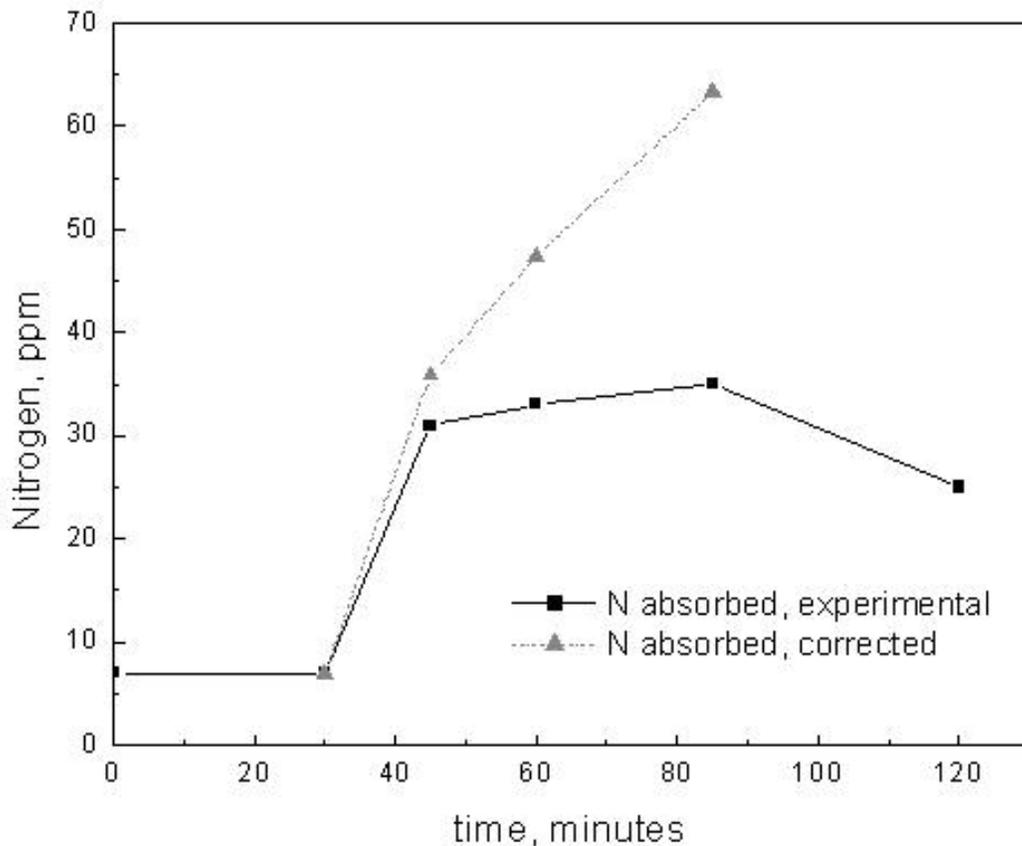
Figure 11, Nitrogen pickup corrected for the desorption, Trial 4
