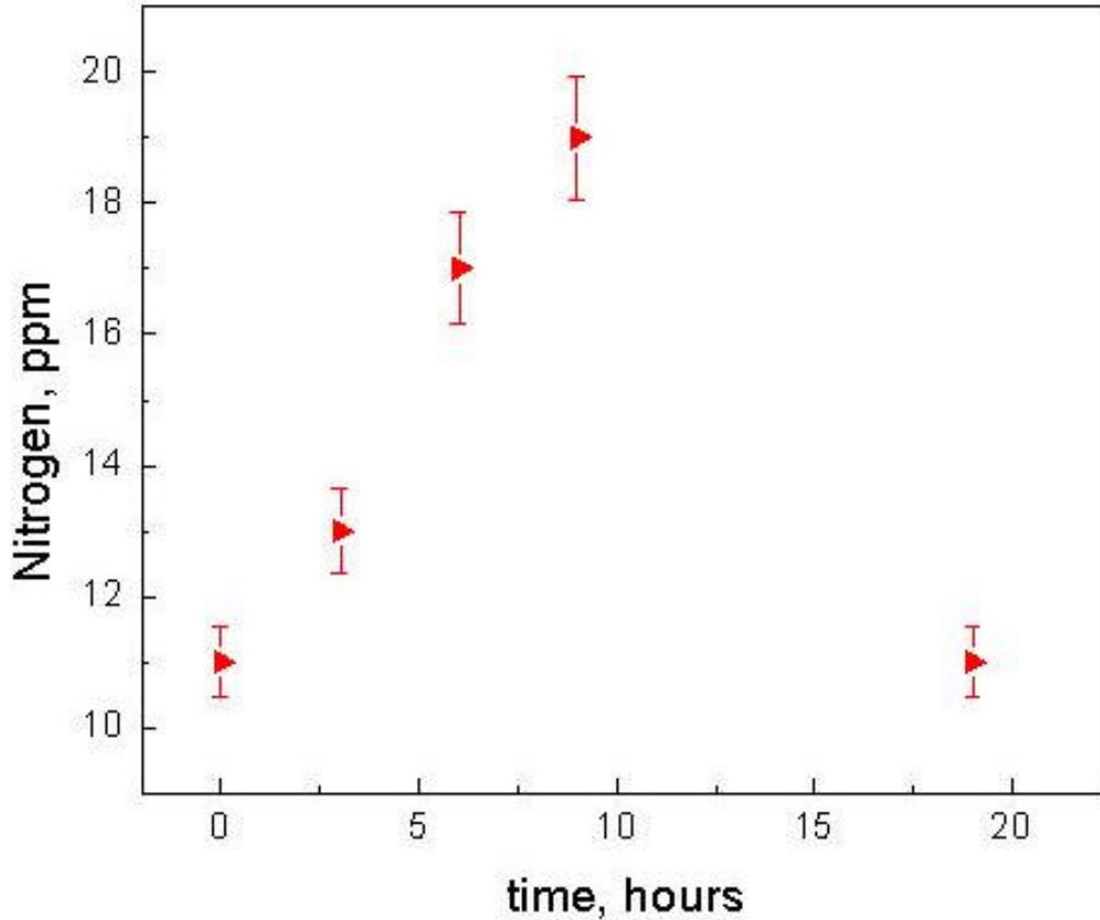
Figure 16, Nitrogen transport through an  $Al_2O_3$  rich slag, Trial 4
