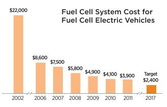
Note: Assumes an 80kw fuel cell system and production of 500,000 units per year. Costs projected based on lab-scale advances. Source: U.S. Department of Energy
