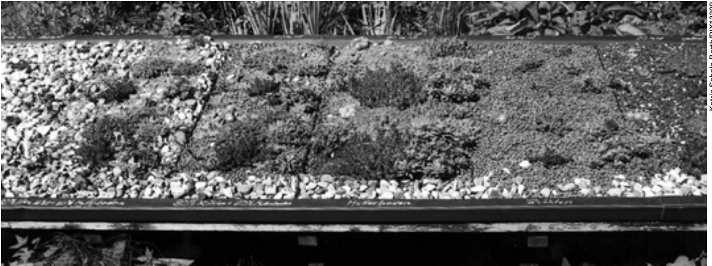
It is important to select the right growing media for a green roof. Selection criteria depend on the intent and desired performance of the green roof. The photo shows, from left, plant establishment in 100 percent gravel, an 80/20 mix of gravel and topsoil, a 20/80 mix of topsoil and expanded clay, 100 percent topsoil, 100 percent expanded clay, and a mix of compost, clay, and sand.
