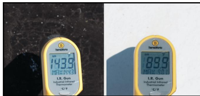
Figure 1: Dark vs. Cool Roof Surface Temperatures
