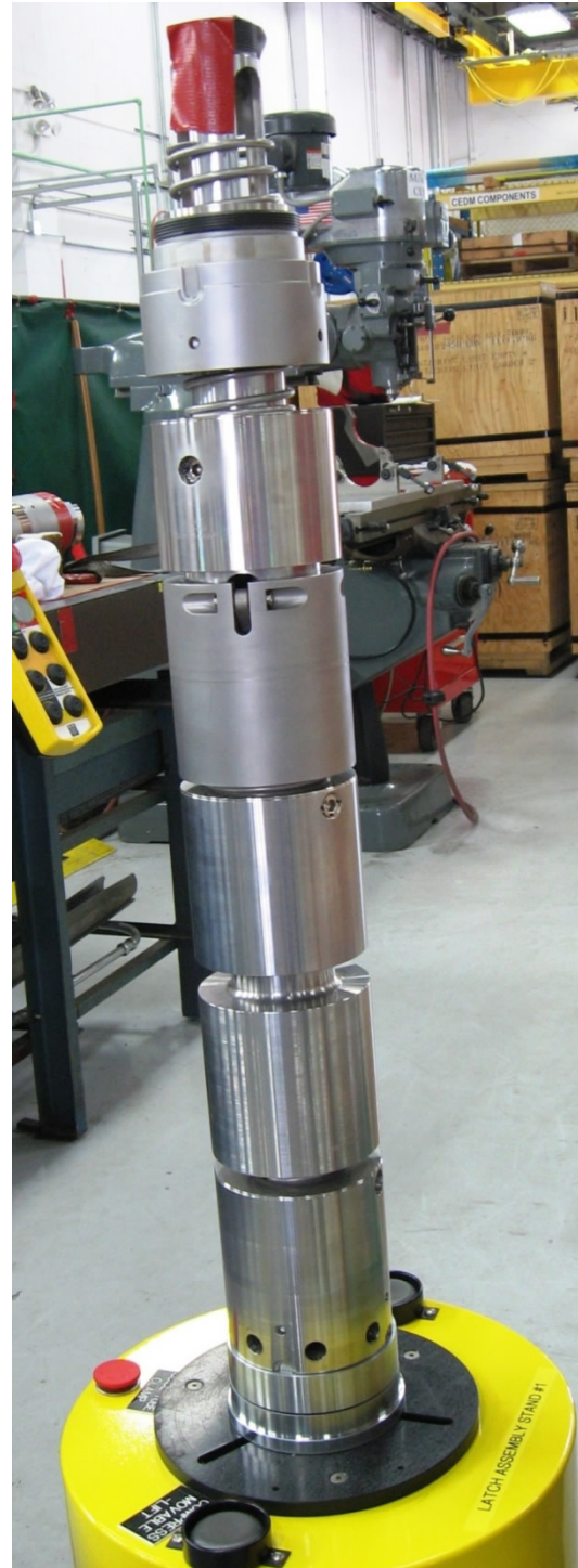
Figure 8. Manufacture of AP1000 Control Rod Drive Mechanism in Newington, New Hampshire
