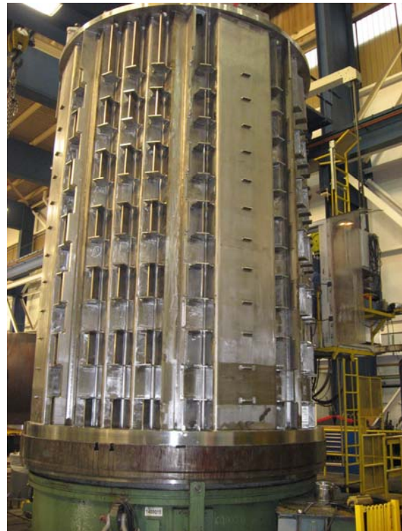
Figure 5. Machining of AP1000 Core Shroud in Newington, New Hampshire
