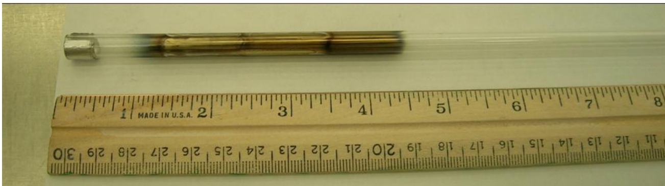
TiN Inner coating formed on glass tube to test TiN coating process
