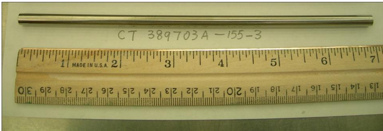
TiN Inner coating formed on glass tube to test TiN coating process
