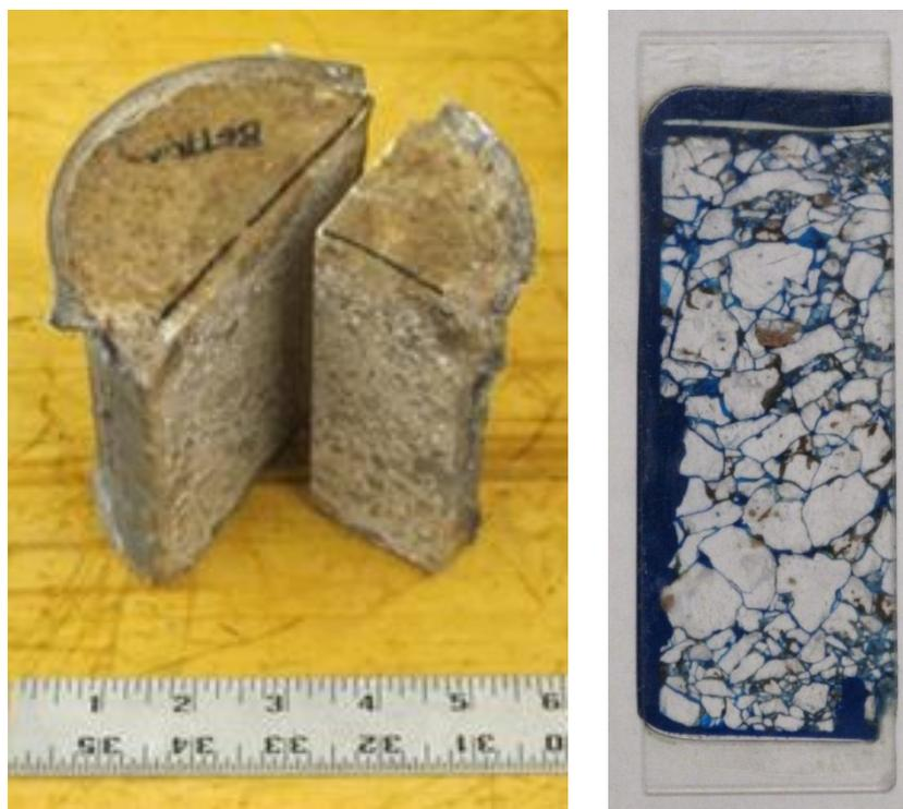
**Figure 4-4. Sawn Samples and an Optical Thick-Thin Section**
