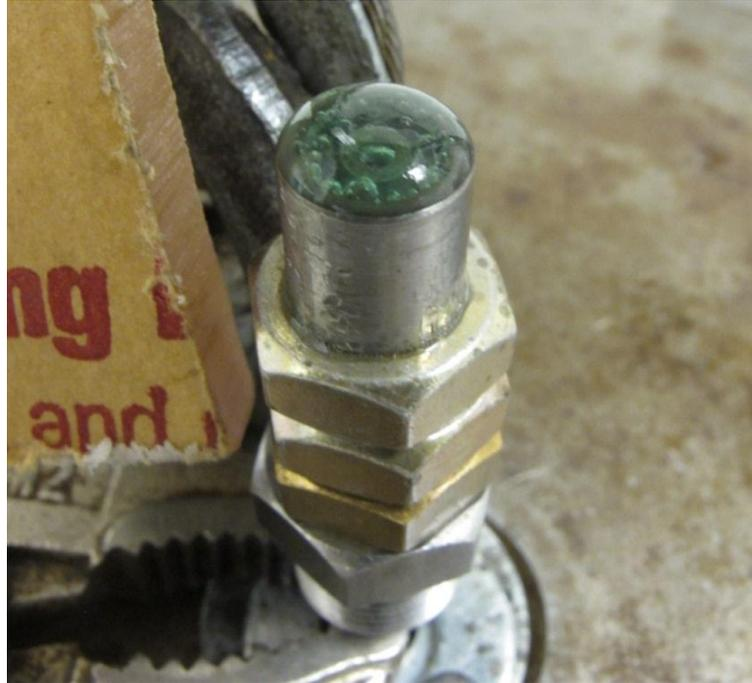
**Figure 2-6. Brine Exiting the Pore Pressure Port at 250°C.**
