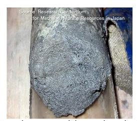
A sand core containing methane hydrate which fills its pore. The core was sampled at eastern Nankai trough
