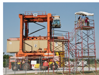
On-dock Rail, which scans cargo containers for radiation, in testing at SRNL
