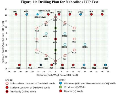
will be placed in the tubing-casing annulus to minimize thermal losses during leaching. All of the wells will be drilled prior to initiation of the 6-9 month leaching phase. Most surface facilities will also be constructed prior to leaching, with only minimal facility conversion required as the project moves into the 2 year pyrolysis and production phase.
