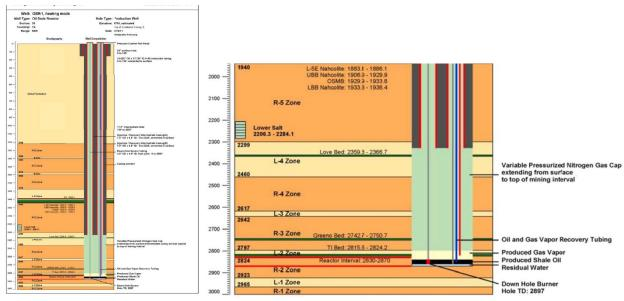
Figure 18. Natural Soda Planned Well Completion Shown During Production Phase
